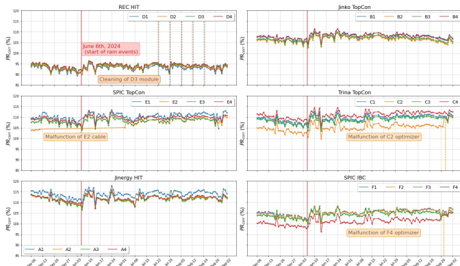
Figure 3 Daily averaged PR_{corr} of each module in installation. Indicated are the start of rain events as well as periods where there were connection issues.
