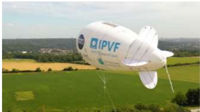
Photography of the airborne platform flying near the SIRTA atmospheric research laboratory inside the Polytechnic School campus. The balloon inflated with helium is equipped with one flexible PV module on top and embedded electronics (27.06.2024).
