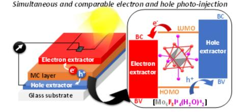
**Transition metal cluster-**based halides are nano-objects that exhibit fascinating optical and electronic properties such as molecule-like energy gaps, strong absorption in the visible or deep red luminescence that make them promising light-harvester for solar energy conversion.<sup>1,2</sup>
